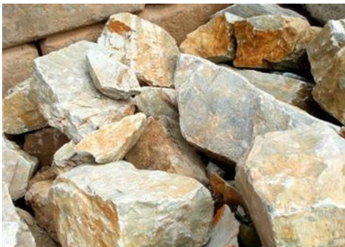
Stone Sample: Glacier/Turquoise Boulder (KRC Rock) Quartzite- light green to dark green in color Sharply angular and irregular
